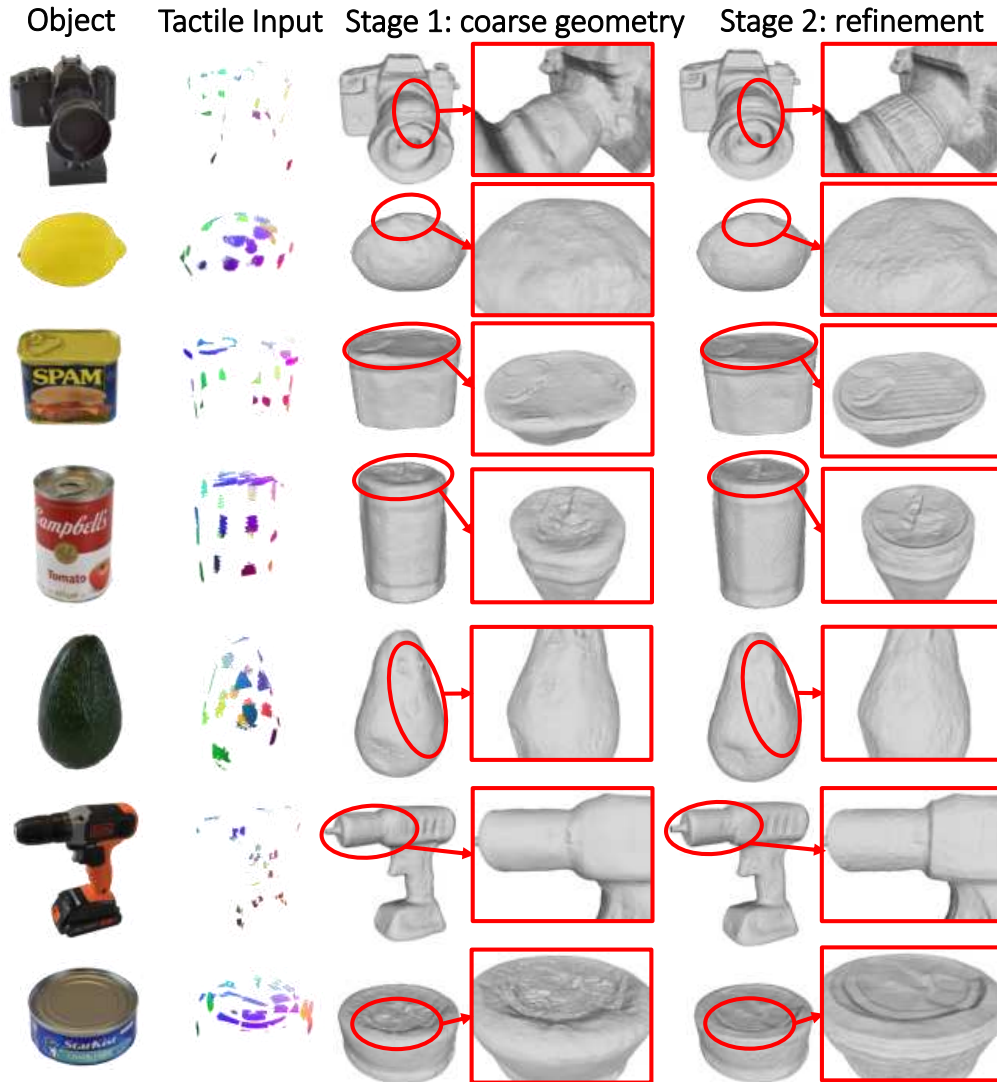
Figure B.4: Qualitative comparison between the results before and after fine geometry learning. We choose some representative objects to show how their surface texture evolves after the stage 2 geometry refinement.
