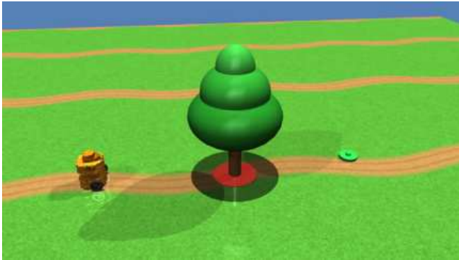
Figure 4.5: The simulation environment. The Dubins Turtle-Bot (orange) must reach the goal region (green ring) while avoiding a single cylindrical obstacle at the origin, rendered as a red disc with a decorative tree on top.
