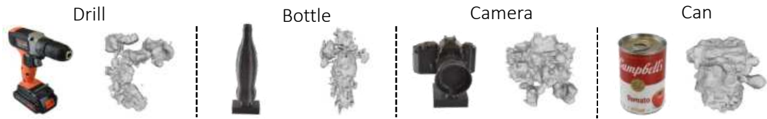
Figure 10.6: Reconstructions using only tactile observations after removing the diffusion prior. The reconstructions degrade significantly.
