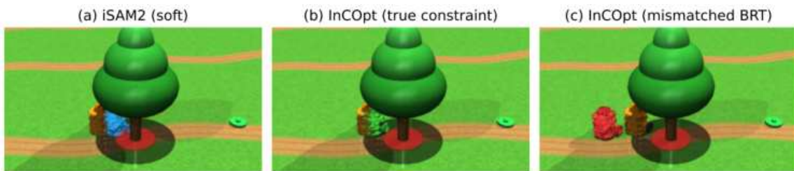
Figure 4.7: Representative estimates under three constraint regimes. (a) The soft iSAM2 baseline enters the obstacle region. (b) InCOpt with the matched BRT keeps the estimate near the safe boundary. (c) InCOpt with the mismatched BRT pushes the estimate farther away from the obstacle than necessary. The orange TurtleBot is ground truth; each transparent ghost is the smoothed estimate at this pose.
